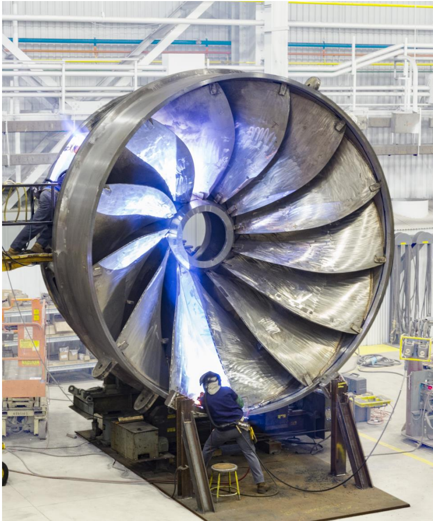
A hydropower turbine being serviced. This turbine is driven by a volume of water which can be adjusted relatively quickly, making it suitable for providing certain grid services.
