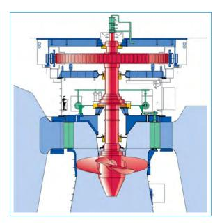
**The Kaplan** is a propeller-type turbine with adjustable blades. It allows for efficient power production in low head applications.
