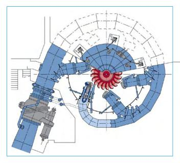
**The Pelton** uses the impulse of water falling in buckets. It is the turbine of choice for high head sites.
